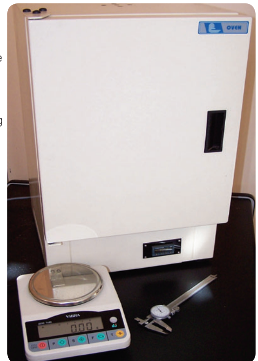
Oven dry testing provides the most accurate moisture content test.
