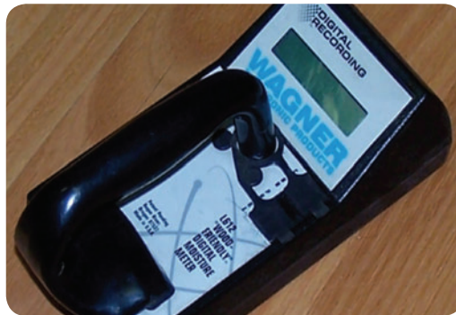
Capacitance moisture meter measures average moisture content. Need to set species density.
