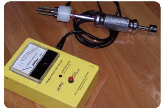
Resistance moisture meter – measures moisture content between the pins. Need to correct reading for temperature and species.
