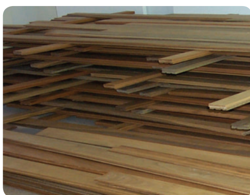
Acclimatisation can be effective if product moisture content and in-service conditions are known.
